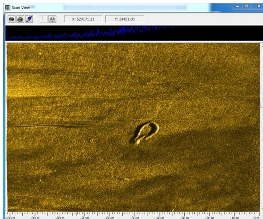
Figure 8: Side Scan Sonar Showing Anchor Pile
