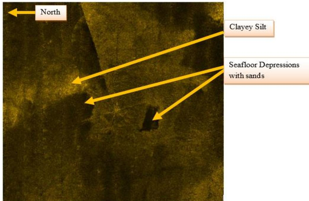
**Figure 2:** Multibeam imagery of seafloor depressions caused by rig movements
