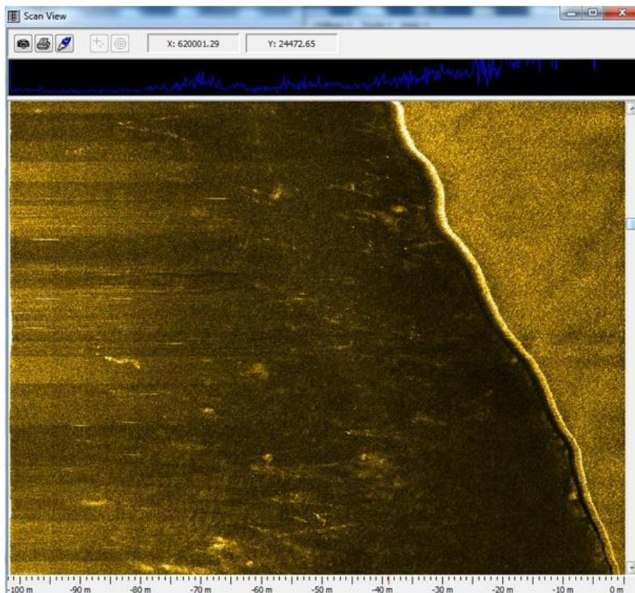
Figure 9: Side Scan Sonar Showing Exposed 42'' pipeline
