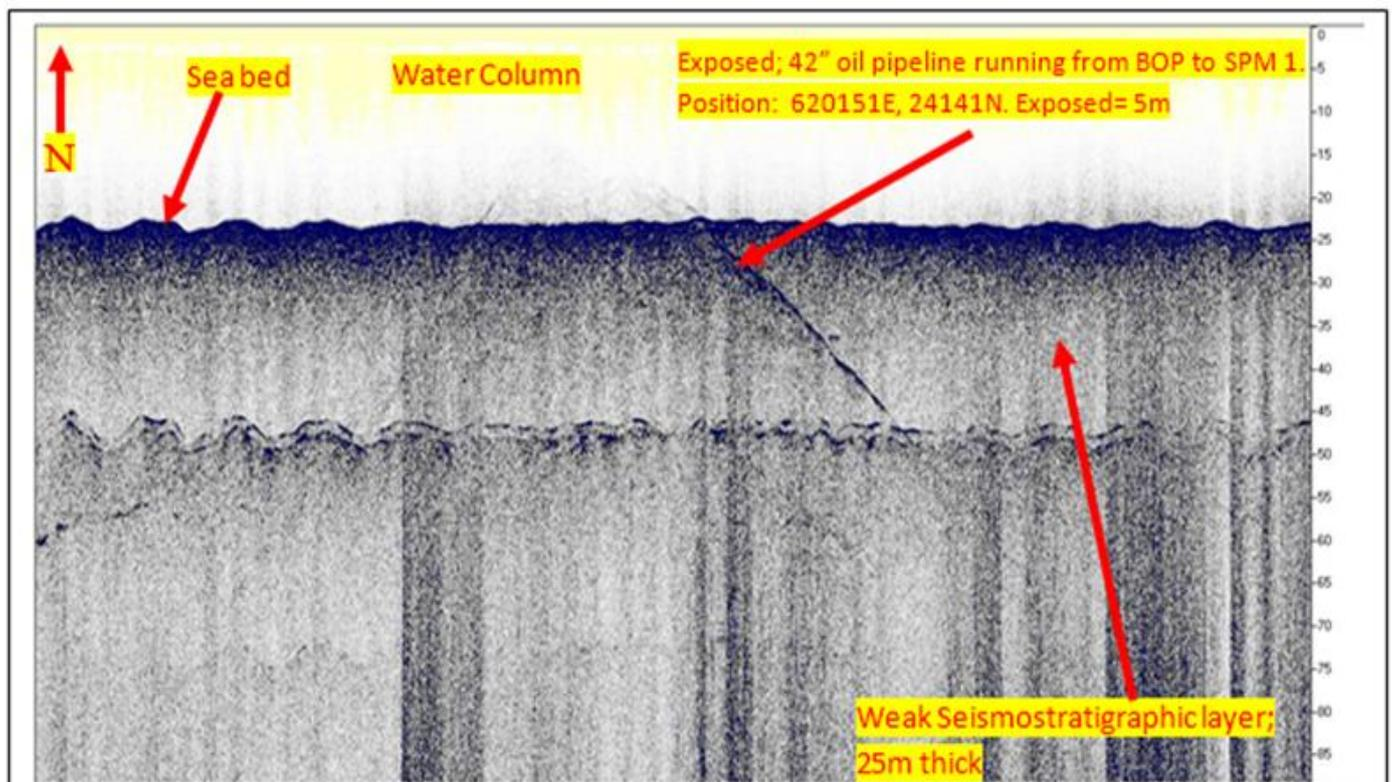
Figure 4: Sub bottom Profile Data Extract Showing the Strata below the Seafloor.
