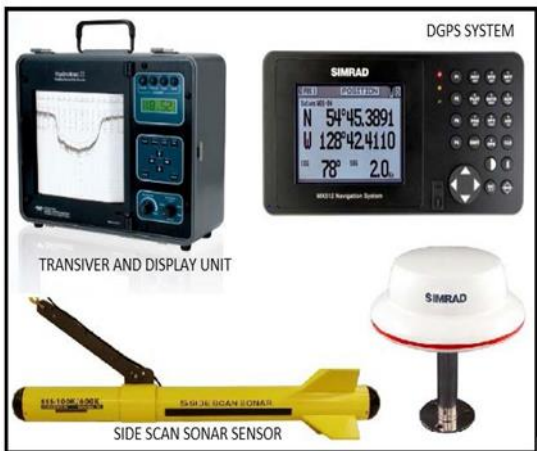
Side Scan Sonar (SSS) System Setup
