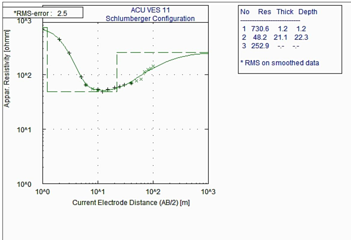
Figure 4(a): H type (VES 11)- Terminates on fractured bedrock
