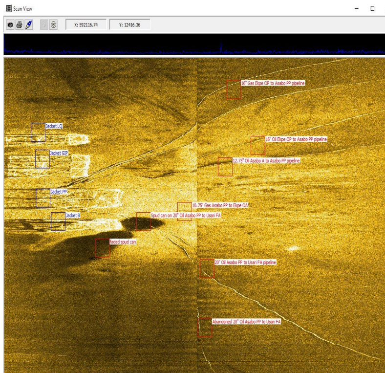
Figure 11: Screen Shot showing Mfotu B, PP, GIP, LQ Jackets, 16" Gas Mfotu OP to Mfotu PP, 16" Oil Ekpe OP to Mfotu PP, 16" Oil Mfotu OP to Mfotu PP, 12.75" Oil Mfotu A to Mfotu PP, 20" Oil Mfotu PP to abandoned 20" Oil Mfotu PP to FA pipelines and spud cans
