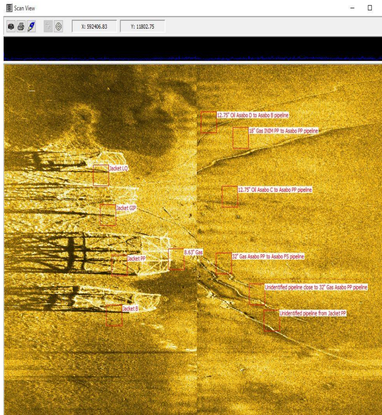
Figure 10: Screen Shot showing Mfotu B, PP, GIP, LQ Jackets, 12.75" Oil Mfotu D to Mfotu B, 18" Gas INIM PP to Mfotu PP, 12.75" Oil Mfotu C to Mfotu PP, 8.63" Gas Mfotu GIP to Mfotu C, 32" Gas Mfotu PP to Mfotu FS, Unidentified pipeline close to 32" Gas Mfotu PP and Unidentified pipelines.
