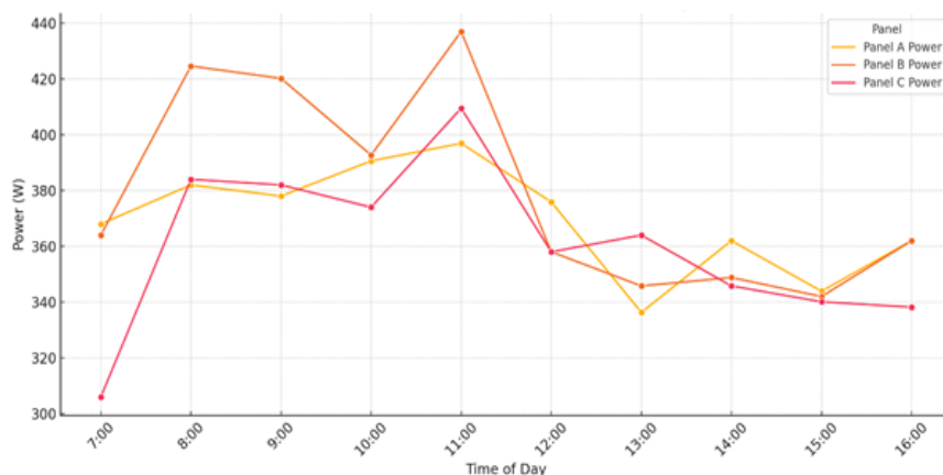
Figure 7: Comparison of the power output for Panels A, B, and C on Day 1.
