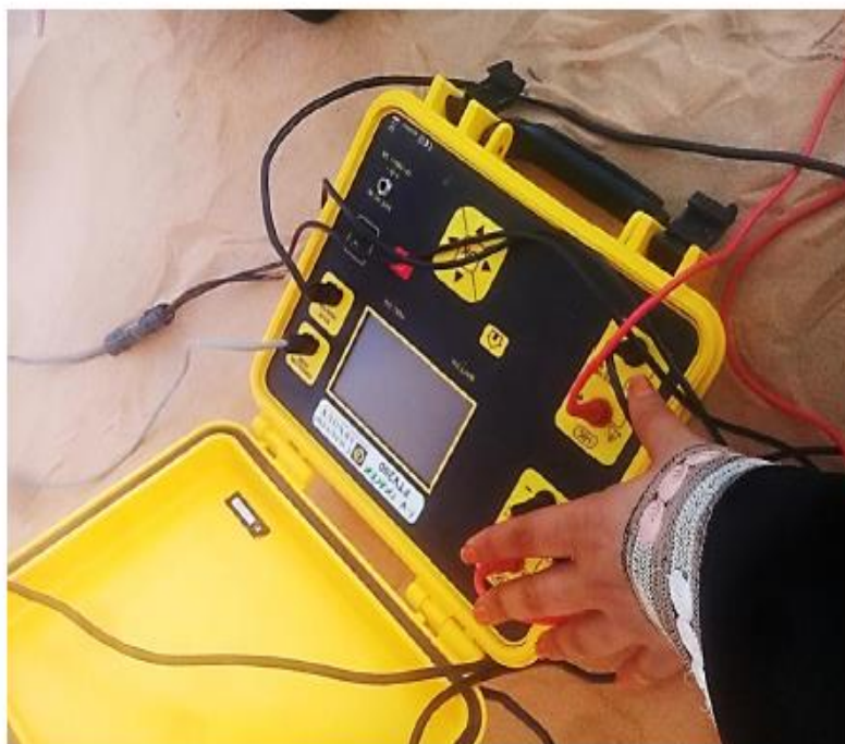
Figure 5. Tracer I-V FTV200 [20].
